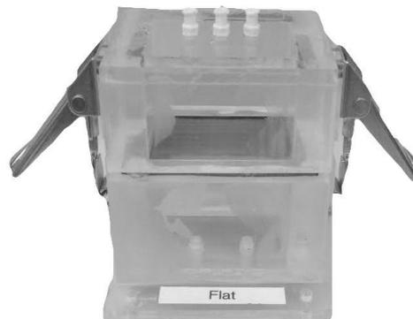
**Figure 7. Picture of the actual flat-screen nominal testing cell. The latches**
